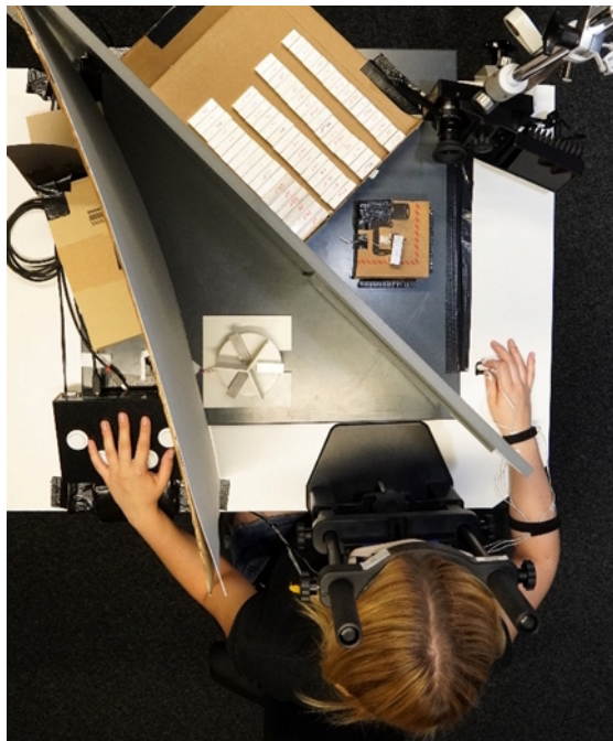
Figure 3: Setup for experiment 2. Participants had their head in a head rest and wore LCD goggles to prevent vision between trials. On any given trials, participants saw one of the objects on the rotating disc in the mirror and grasped an object behind the mirror that was in the same location the visual object was projected to. The eye tracker registered gaze position and pupil dilation through the cold mirror. Grasping movements were registered through diodes on the thumb, index finger and wrist, as well as one next to the haptic object that was placed such that it was visible to the 3D-Investigator when the reflective side of the object was next to it, but not visible when the object was moved, thus serving as a marker of object touch.
